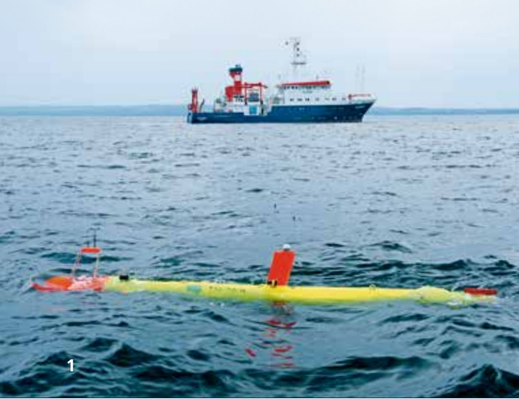
1 Deep-sea AUV TIETEK and research vessel ALKOR during a test run in the Baltic Sea.
